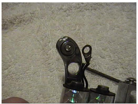
You should put a washer both in front of and behind the connector loop for the contact post.
