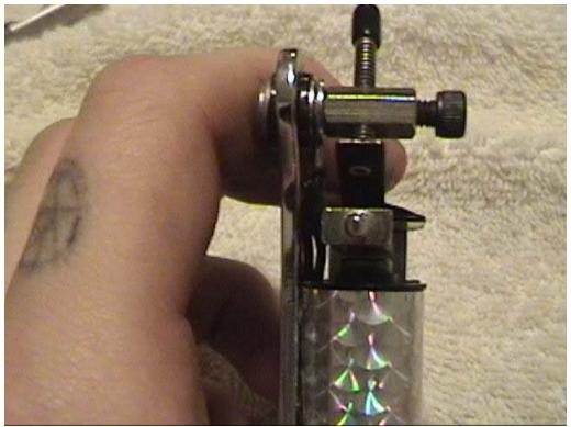
Notice in this image the armature bar is too far to the left although the contact spring is aligned. This will cause an abnormal wear pattern on the bottom of the armature bar.
