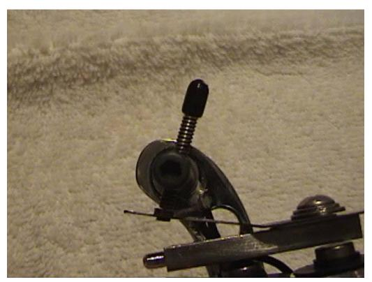
From the side, make sure the contact spring and screw line up..round off the end of the contact spring for a better fit and connection.
