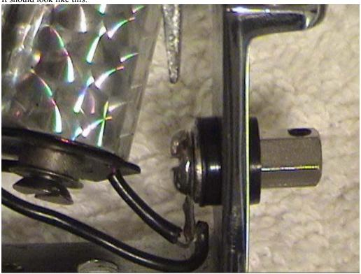
Now you have to line the coils up on the frame like such, making sure not to pinch any wires, snug them both down making them as even and squared as possible.
