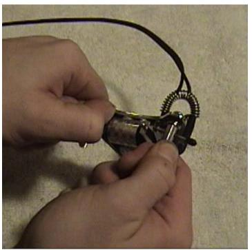
By the way, I must add that there should be a tiny nylon bead inside your stop screw hole between your contact screw and the stop screw, this keeps it snug without bending the threads of your contact screw or ruining the end of a nylon screw. Most tattoo suppliers stock them, although I've noticed more than my share of tattooists that do not use them.
