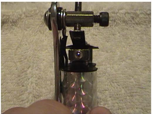
Notice in this image that the contact spring is off-center from the armature bar, yet it is aligned with the contact screw and the armature bar aligned with the tops of the coils-this is the correct position. Not every machine will tune off-centered like this, but it is best to illustrate this possibility to assure you that even if it looks funny like this, this is the correct position.
