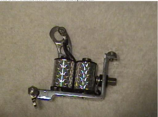
This is temporary so do not over tighten, but they need to be snug and not loose at all. Go ahead an bend the wires so they are in their best positions -like this:
