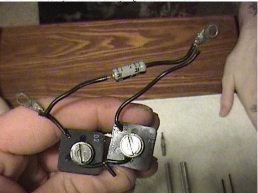
The capacitor in this picture is a 35mf, however you can use up to 150mf, I would suggest using between 75-100mf personally.
