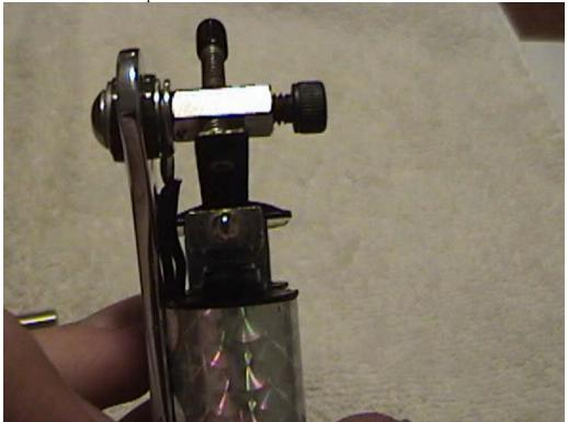
It this image, notice that the armature bar is aligned, but the contact point on the contact spring is off-centered to the right of the contact screw...this is also incorrect and will wear down the points on both the screw and the spring in an awkward manner.
